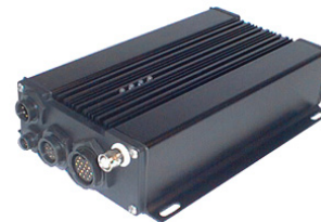
Figure 6: Smart digital controller measures signals and processes data, independent of PC, with internal digital relay outputs.
