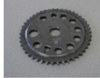
Figure 8: Powdered metal sprocket.
