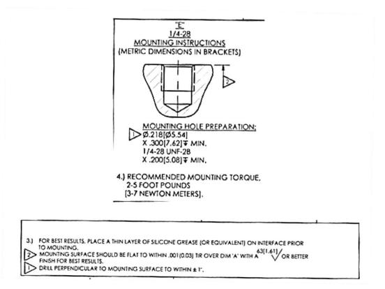
Figure 2: Mounting Surface Installation Drawing
