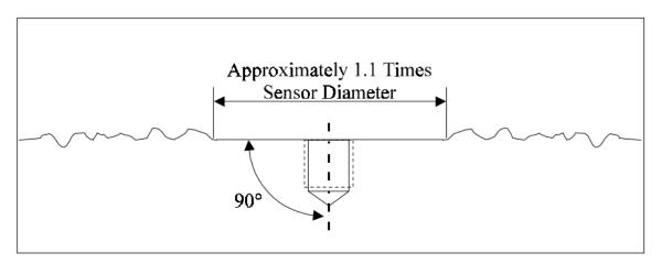
Figure 1: Mounting Surface Preparation
