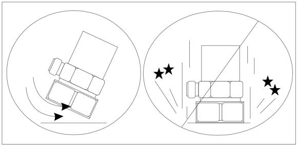
Figure 5: Magnet Mounting
